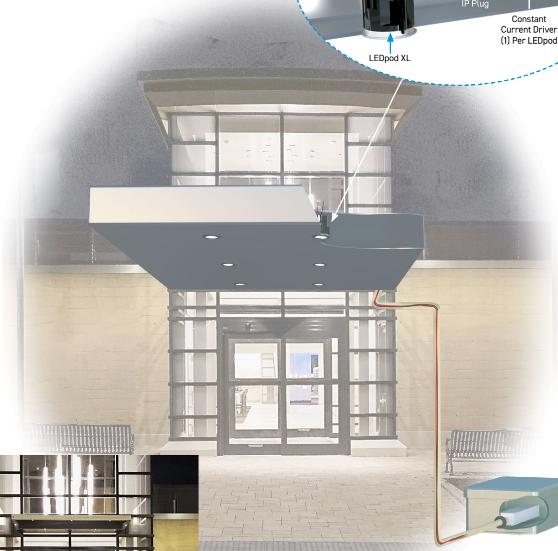
24VDC Wiring to railing via conduit; from constant voltage primary driver in remote enclosure
