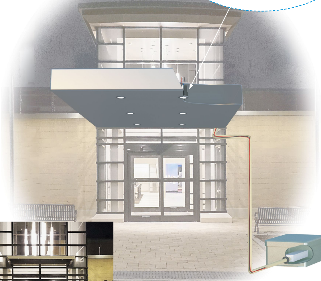
24VDC Wiring to railing via conduit; from constant voltage primary driver in remote enclosure
