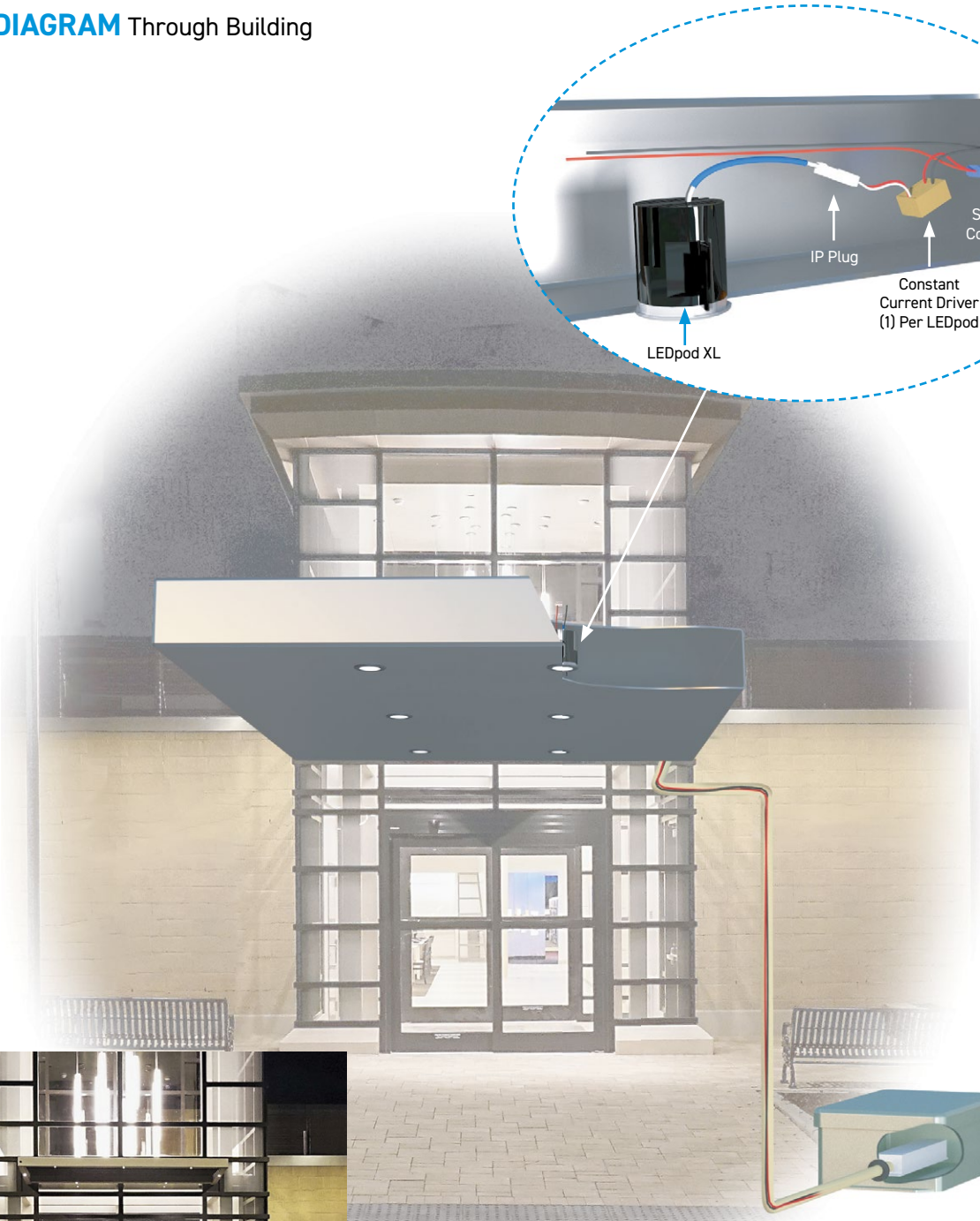
24VDC Wiring to railing via conduit; from constant voltage primary driver in remote enclosure
