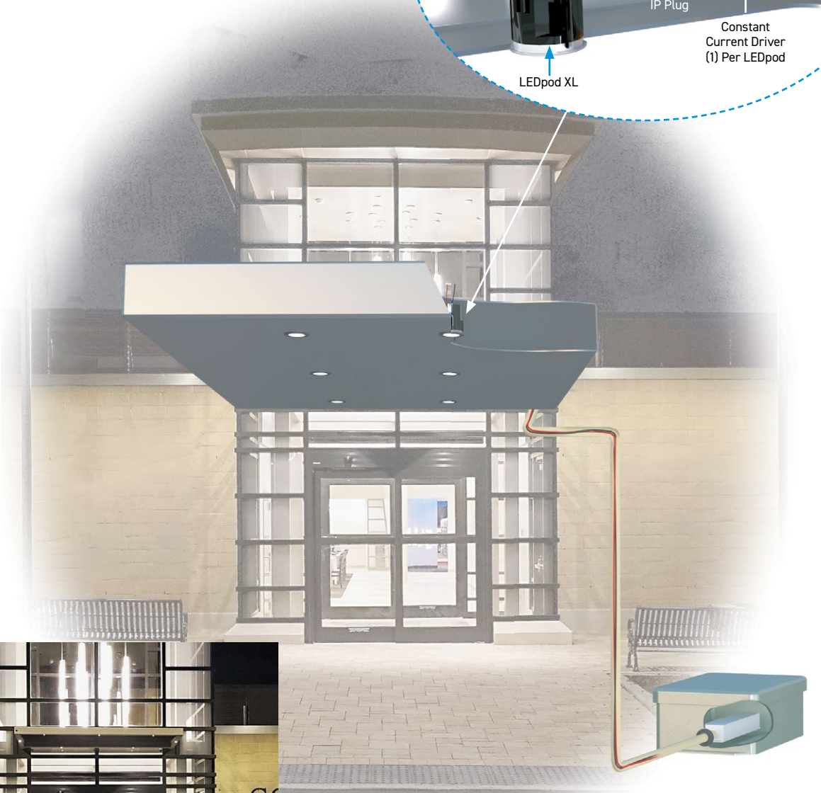
24VDC Wiring to railing via conduit; from constant voltage primary driver in remote enclosure
