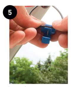
Secure Scotch-Lok connector to through-wire, then insert transformer wire into second hole.
